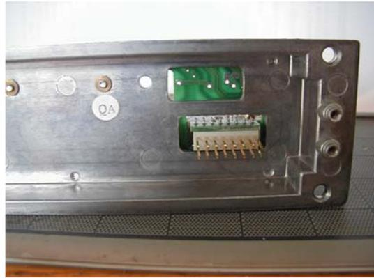
The above illustrates a radio without memory backup battery fitted
